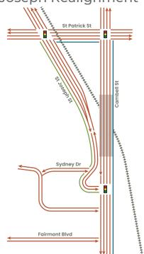
This alternative would eliminate the existing on/offramps that connect St. Joseph Street and Cambell Street. St. Joseph Street and Bridge View Drive would be merged into a continuous alignment, and a new traffic signal would be added to the intersection of Cambell Street and St. Joseph Street. Sidewalks would be added to Cambell Street and St. Joseph Street/Bridge View Drive.
