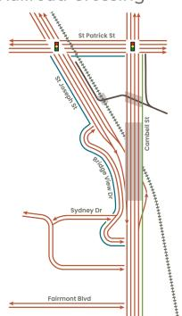
would adjust the alignment of St. Joseph Street to cross the railroad (at-grade or via a structure) and intersect with Cambell Street at a 90-degree angle south of the existing warehouse facility at 1313 St. Patrick Street. A traffic signal would be installed at the new intersection of St. Joseph Street and Cambell Street, with sidewalks added to Cambell Street and St. Joseph Street
